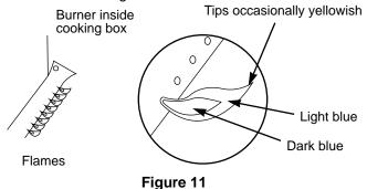
If the flames do not appear to be uniform the length of the burner tube, follow the burner cleaning procedures.
